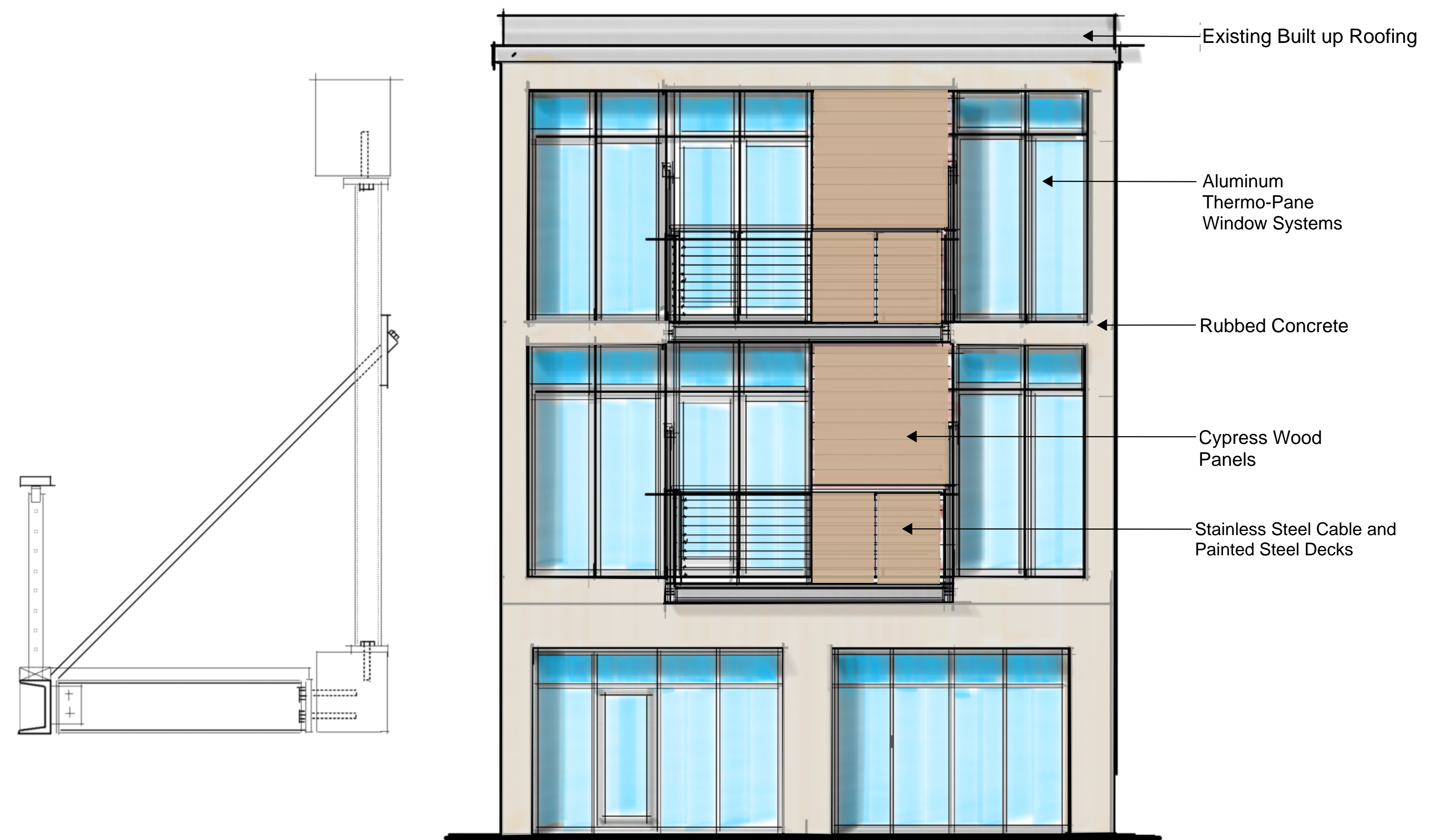
TYPICAL EXTERIOR IMPROVEMENTS NO SCALE
