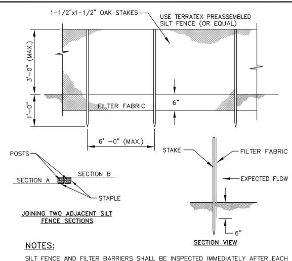
SILT FENCE AND FILTER BARRIERS SHALL BE INSPECTED IMMEDIATELY AFTER EACH RAINFALL AND AT LEAST DAILY DURING PROLONGED RAINFALL. ANY REQUIRED REPAIRS SHALL BE MADE IMMEDIATELY.
