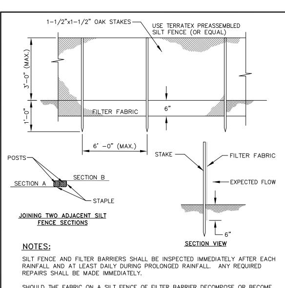
SHOULD THE FABRIC ON A SILT FENCE OF FILTER BARRIER DECOMPOSE OR BECOME INEFFECTIVE PRIOR TO THE END OF THE EXPECTED USABLE LIFE AND THE BARRIER STILL IS NECESSARY, THE FABRIC SHALL BE REPLACED PROMPTLY.
