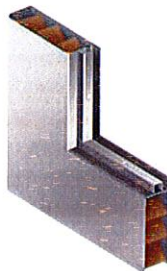
DLF flush vision kit , 16-gauge (0.056"/1.4 mm). Spot welded, available for 1/4" (6.3 mm) to 1" (25.4 mm) thick glass (P series).
