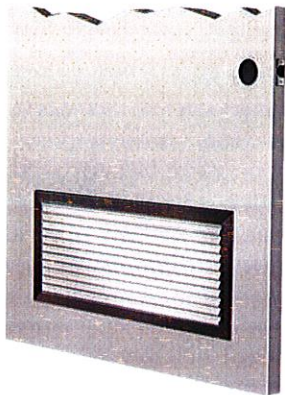
Standard two-part sandwich-type louver , inverted "Y" blades, welded corners, 50% free-flow area, 18-gauge (0.044"/1.1 mm). Available in CRS, A40, A60 material and fire rated.
