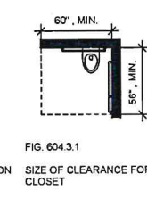
FIG. 604.3.1 - SIZE OF CLEARANCE FOR WATER CLOSET
