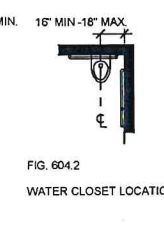
FIG. 604.2 - WATER CLOSET LOCATION
